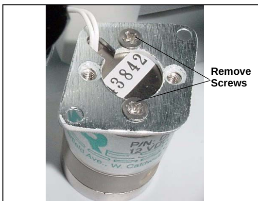
Figure 5-26. Removing the Valve Mounting Plate
