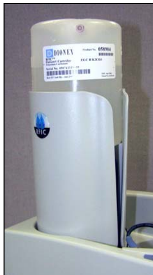
Figure 5-48. EluGen Cartridge Installed in the Holder
