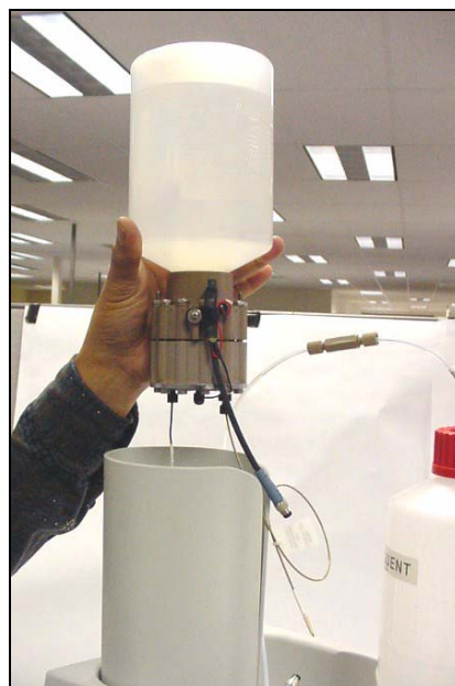
Figure 5-38. Installing the EluGen Cartridge in the Holder
