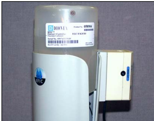
Figure B-62. EPM and Mounting Bracket Installed on EGC Holder
