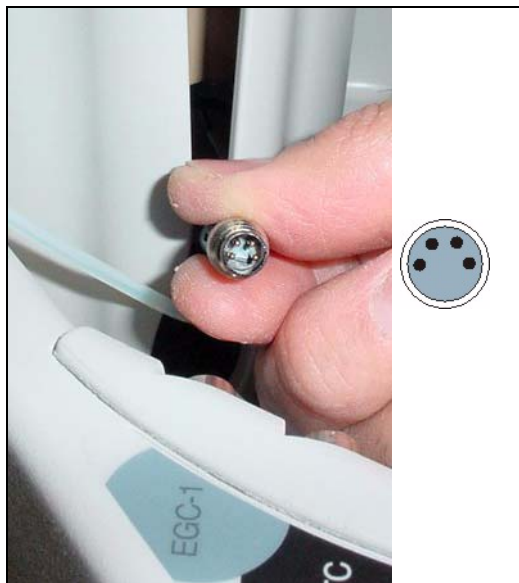
Figure B-58. Connecting the EluGen Cartridge Cable
