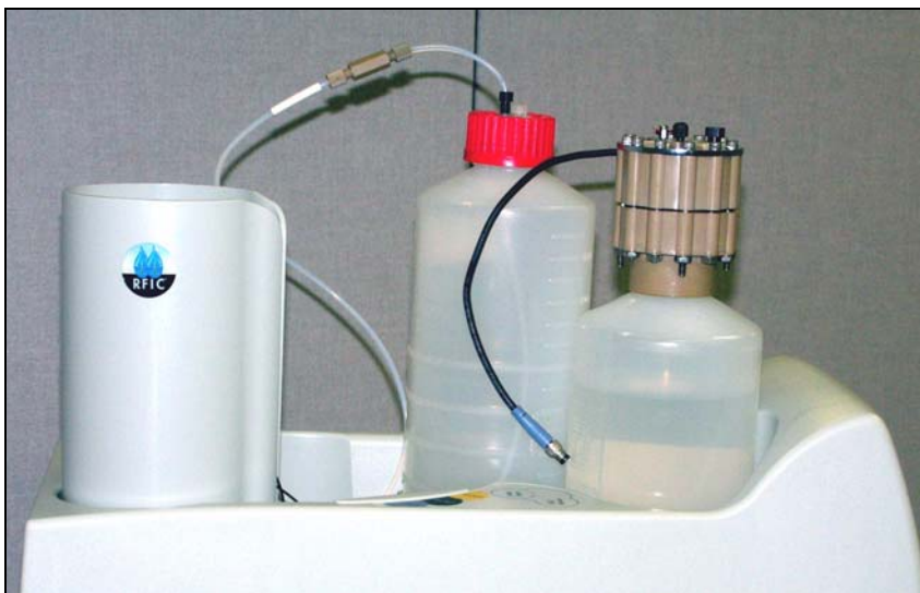
Figure B-38. EluGen Cartridge in Service Area
