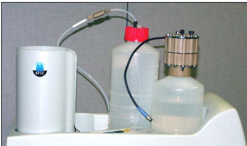
Figure B-79. EluGen Cartridge in Service Area
