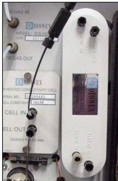
Figure B-23. Suppressor Installed (SRS Shown)
