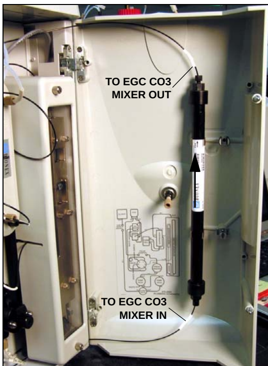
Figure 5-62. ICS-2000 with an EGC CO 3 Mixer Installed
