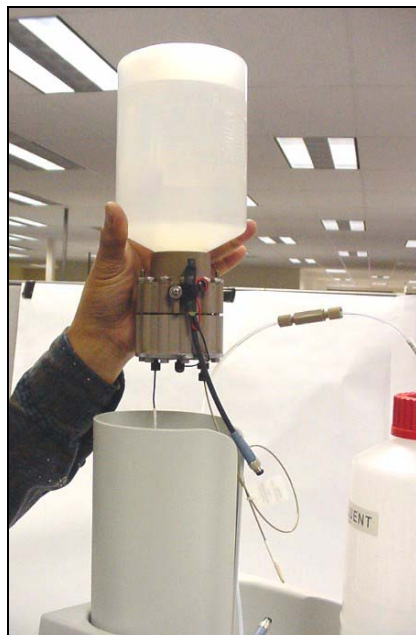
Figure B-41. Installing the EluGen Cartridge in the Holder
