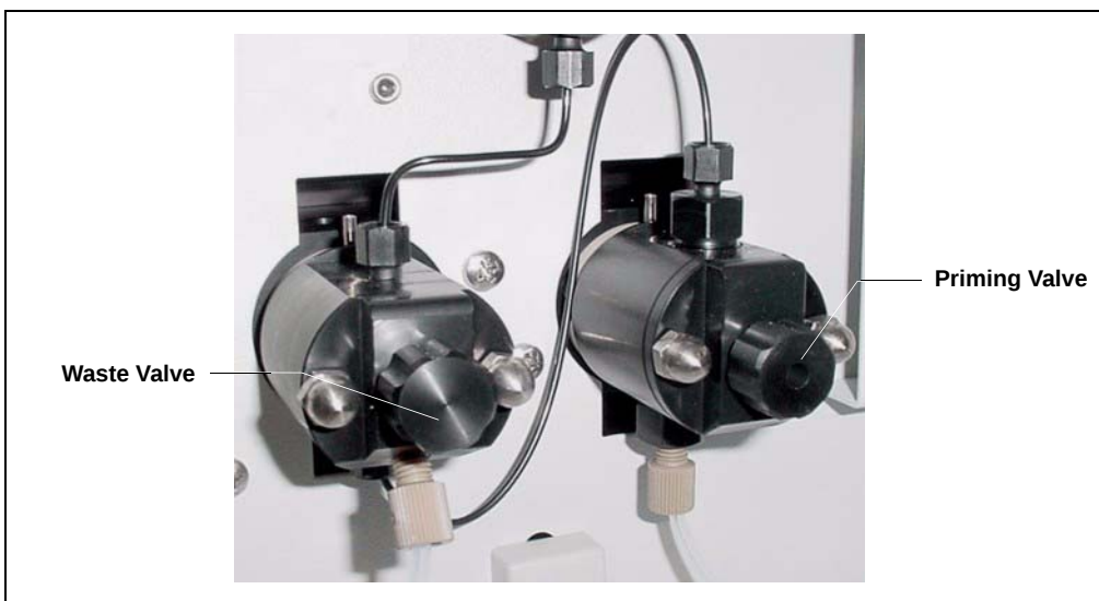
Figure 5-14. Waste and Priming Valves
