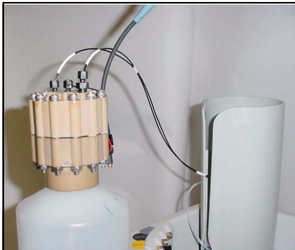
Figure B-46. EGC Inlet and Outlet Connections
