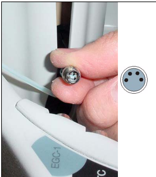
Figure B-82. Connecting the EluGen Cartridge Cable
