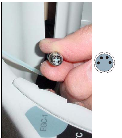
Figure B-42. Connecting the EluGen Cartridge Cable
