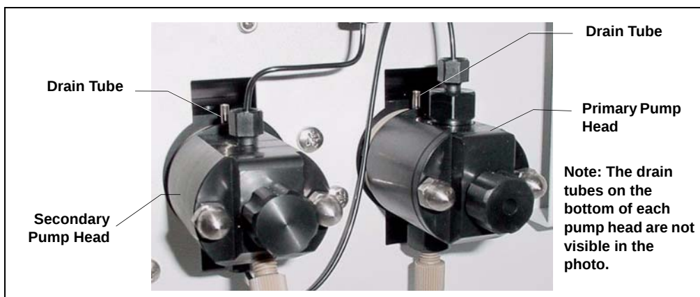
Figure B-113. Primary and Secondary Pump Heads with Drain Tubes
