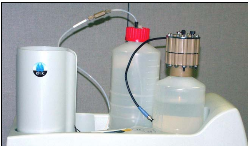
Figure B-55. EluGen Cartridge in Service Area
