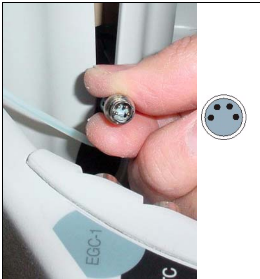
Figure 5-39. Connecting the EluGen Cartridge Cable
