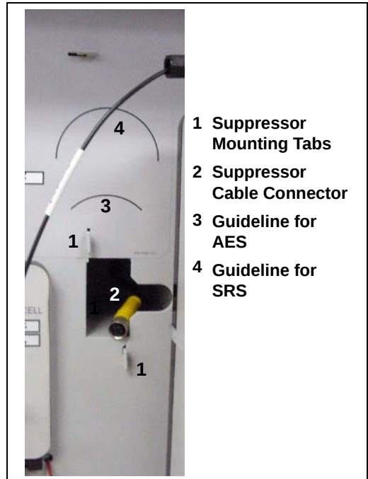
Figure B-22. Suppressor Mounting Tabs and Guidelines
